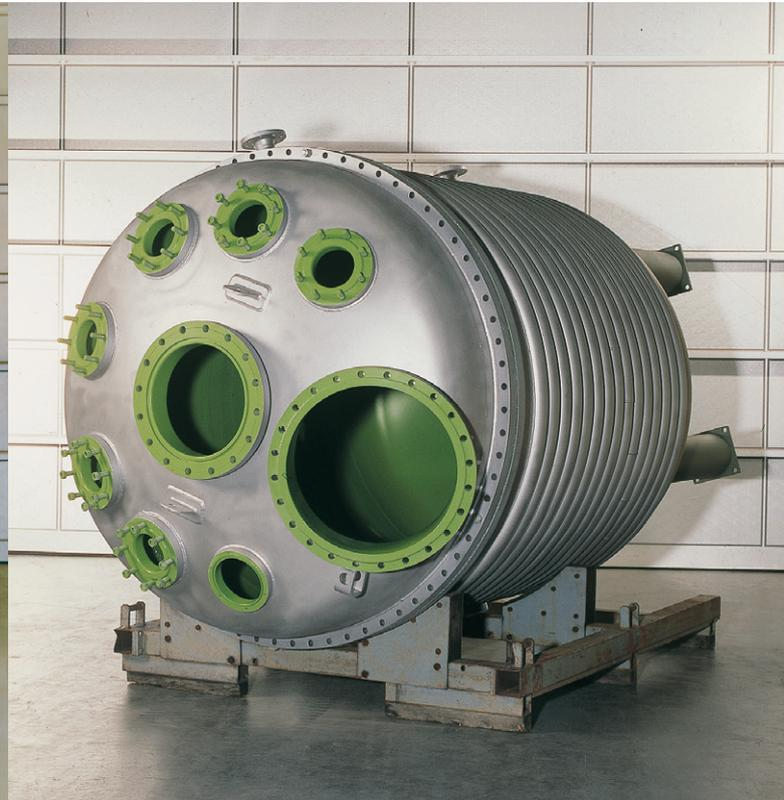
In the spraying sinter procedure (airless and compressed air process), Gutbrod works with Teflon™ Coating. The coating is sprayed on and then „sintered“ at 220°C to 420°C.
