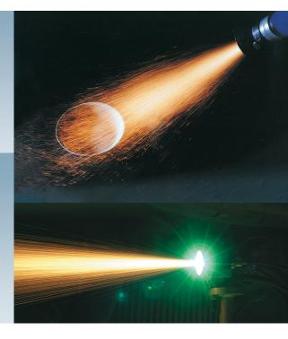
The basis for the Gutbrod combination coatings is a wear-resistant, thermally sprayed hard substrate layer made of metallic material. Using a special flame spraying technique, this is melted on and applied using atomizer gas onto the component surface being treated.
