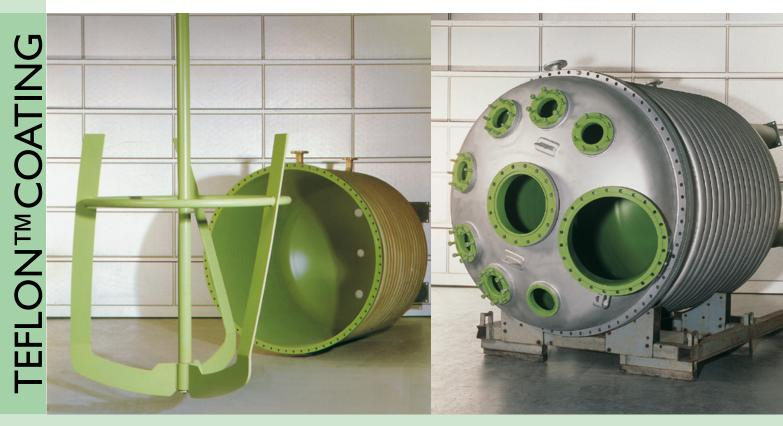
In the spraying sinter procedure (airless and compressed air process), Gutbrod works with Teflon<sup>TM</sup>Coating. The coating is sprayed on and then "sintered" at 220°C to 420°C.
